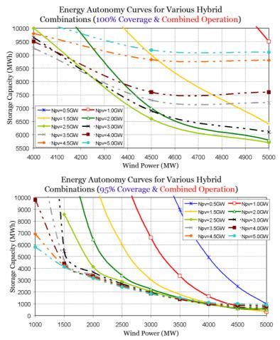
Figure 2. Energy autonomous hybrid combinations that can achieve 100% and 95% coverage of the Ptolemaida-V base load, assuming a 10 GWh upper limit in capacity storage
