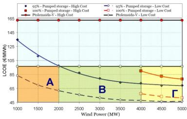
Figure 3. Levelised production cost of energy autonomous hybrid combinations - Achieving 100% (a) and 95% (b) coverage of the base load, assuming a ≤10 GWh storage capacity
